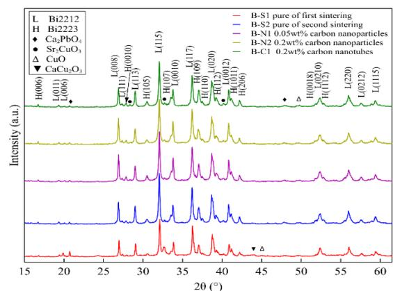
**Figure 1** Diffraction patterns of the pure and carbon added BPSCCO sample prepared by two-step sintering process.
