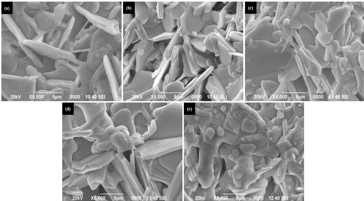
**Figure 2.** SEM images of the pure and carbon added BPSSCO samples (a) pure of first sintering, (b) pure of second sintering, (c) 0.05 wt% carbon nanoparticles, (d) 0.2 wt% carbon nanoparticles, and (e) 0.2 wt% carbon nanotubes added BPSSCO.
