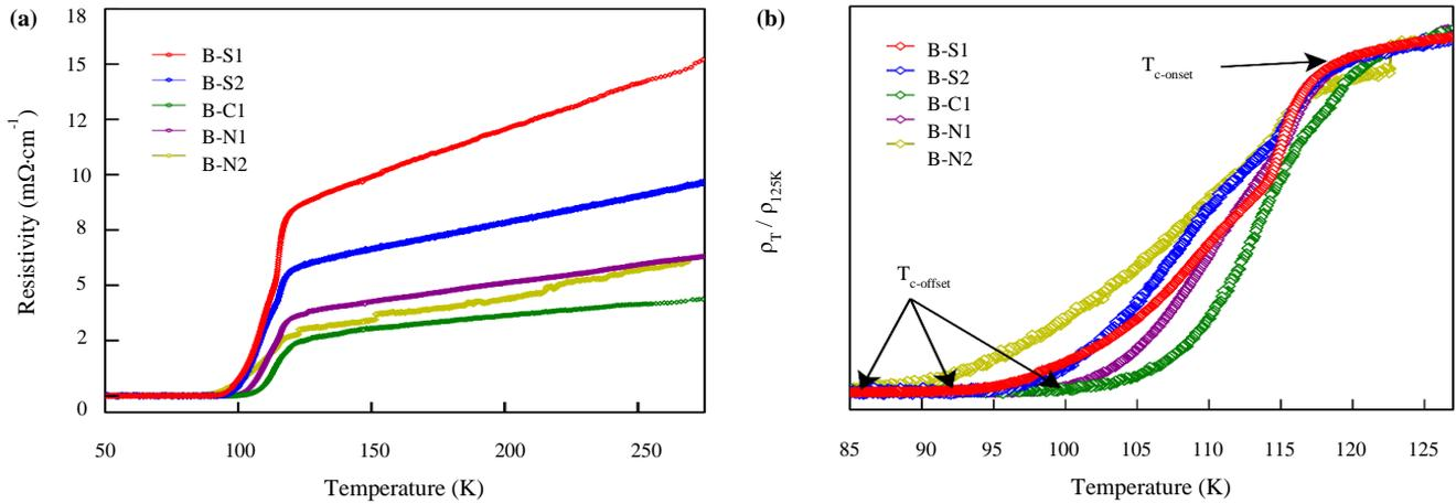
**Figure 3.** Electrical resistivity of the pure and carbon added BPSCCO samples (a) R-T curve, and (b) normalized resistivity vs temperature.
