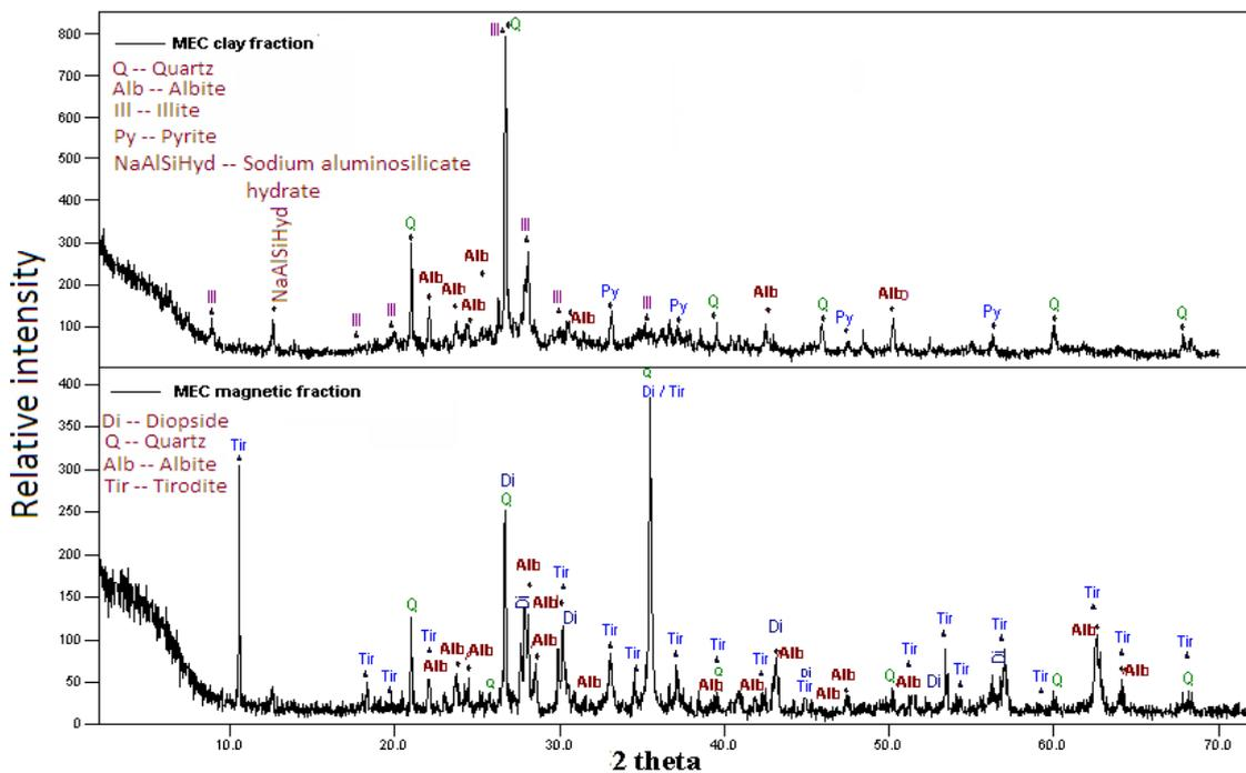
**Figure 2.** X-ray diffractogram for the MEC sample. At the upper figure, we have the one corresponding to the clay fraction; at the lower figure, the one corresponding to the magnetic fraction.
