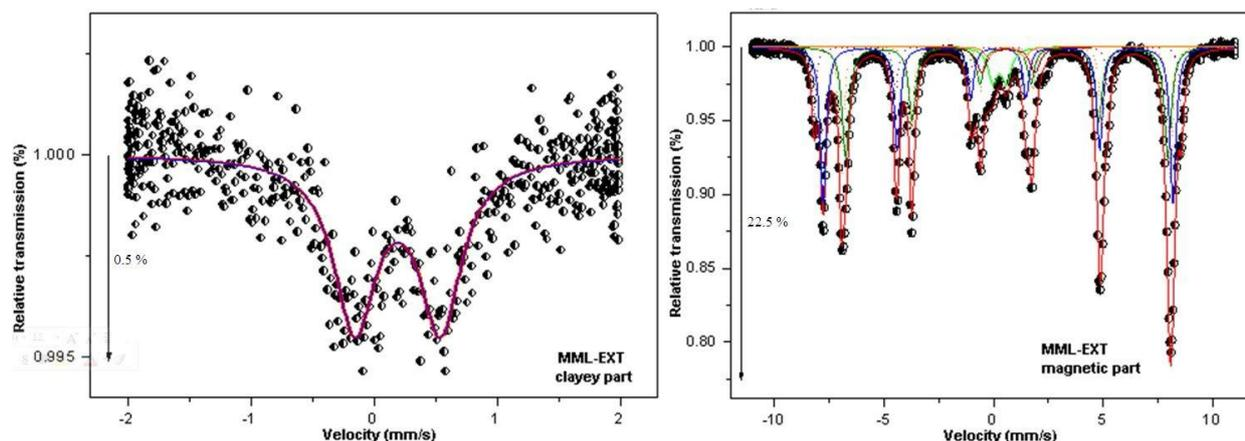
**Figure 3.** Transmission Mössbauer spectrum for the MML-EXT sample corresponding to the clay fraction, recorded at low maximum Doppler velocity  $v_{\max} = 2$  mm/s (left side); and the one corresponding to the magnetic fraction, at velocity  $v_{\max} = 11$  mm/s (right side).
