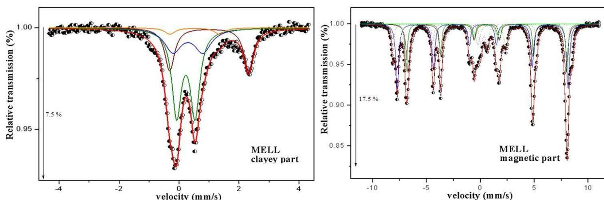
**Figure 4.** Transmission Mössbauer spectrum for the MELL sample corresponding to the clay fraction, recorded at low maximum Doppler velocity  $v_{\max} = 4$  mm/s (left side); and the one corresponding to the magnetic fraction, at velocity  $v_{\max} = 11$  mm/s. (right side).
