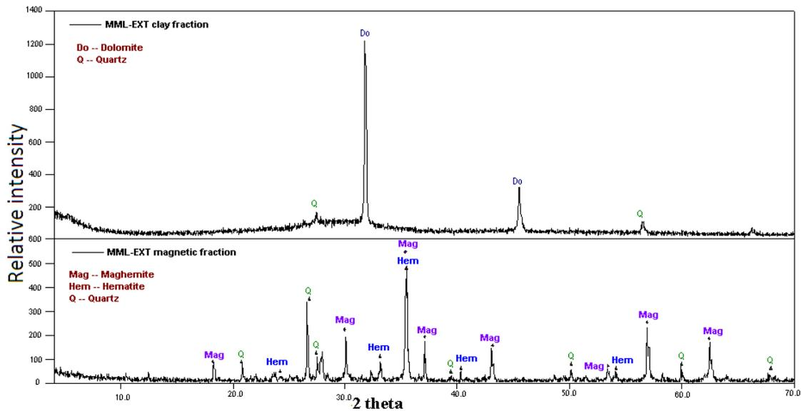
**Figure 1.** X-ray diffraction patterns for the MML-EXT sample. At the upper figure, we have the one corresponding to the clay fraction; at the lower figure, the one corresponding to the magnetic fraction.
