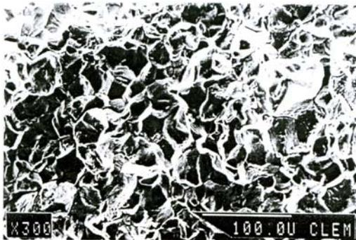
**Figure 6** Crack nucleation and propagation in intergranular fracture
