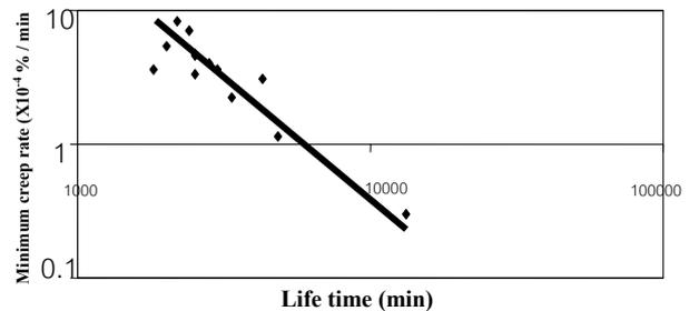
Figure 5 The relationship between minimum creep rate and lifetime
