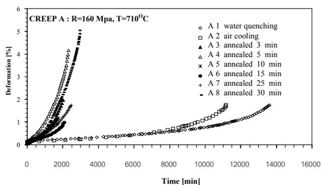
**Figure 1** Creep curves of program A
