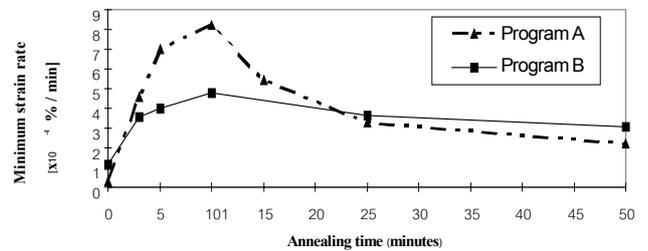
Figure 4 The relationship between minimum strain rate and annealing time
