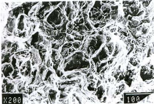
**Figure 7** Mixing mode fracture facet
