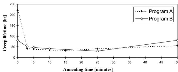
Figure 3 The relationship between creep lifetime and annealing time in program A and B
