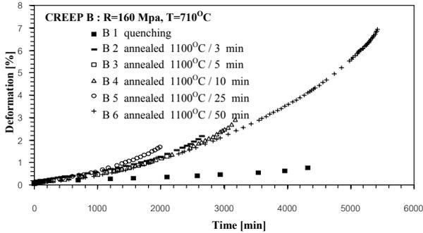
Figure 2 Creep curves of program B
