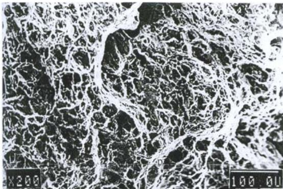
**Figure 8** Crack propagation in transgranular ductile fracture (dimple)
