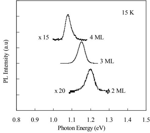
**Figure 4** PL spectra as a function of the well width at 15 K
