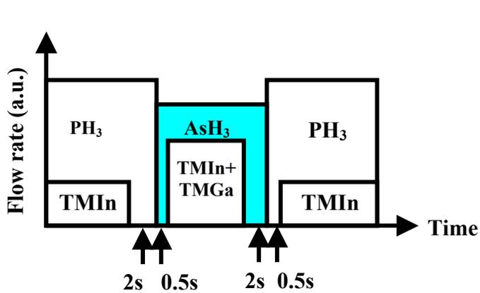
**Figure 1** Flow sequence of gas sources for InP/InGaAs SQWs.
