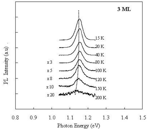
**Figure 6** PL spectra of a 3-ML sample as a function of temperature.
