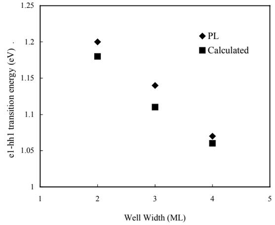
**Figure 5** Transition energy of e(1)-hh(1) in InP/InGaAs/InP SQWs as functions of well width by PL experiment.
