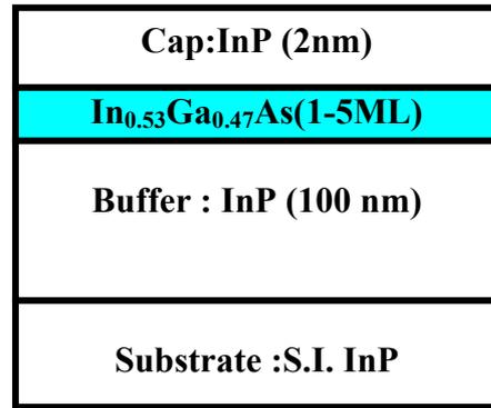
**Figure 2** Sample structure of InP/In<sub>0.53</sub>Ga<sub>0.47</sub>As/InP SQWs.
