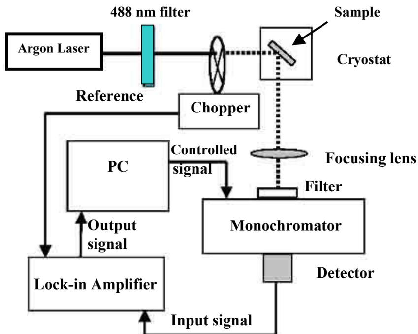
**Figure 3** Schematic diagram of Photoluminescence experiment set up.
