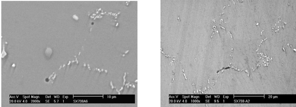
**Figure 2.** As-received microstructure after long-term service showing microvoids
