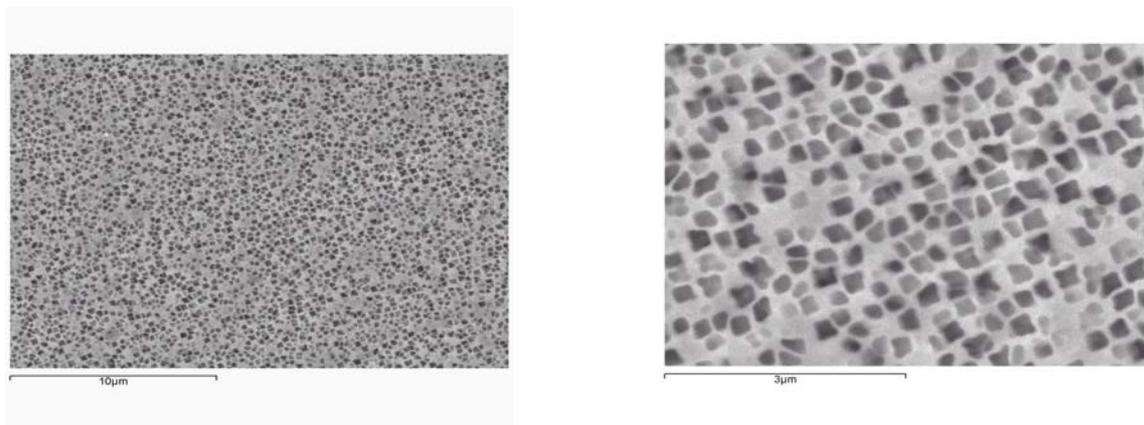
**Figure 5.** After heat-treatment at 925°C / 1 hr. (AC), and 845°C / 24 hr. (AC); Condition No. 2
