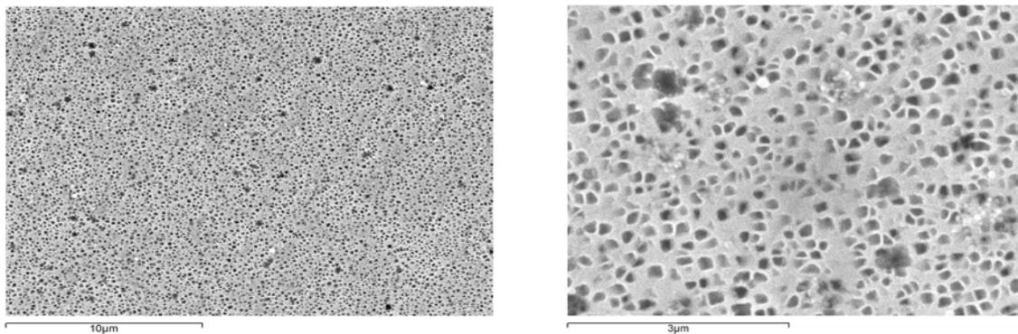
**Figure 3.** HIPed Microstructure showing partial dissolved gamma prime particles
