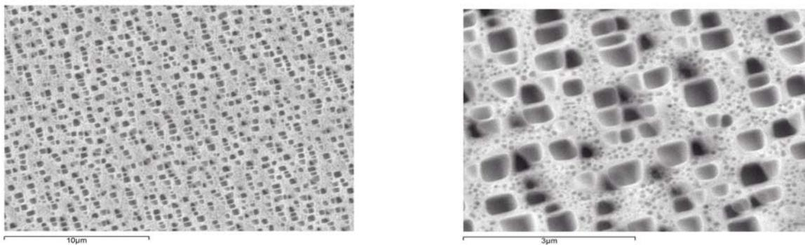
**Figure 9.** After heat-treatment at 1125°C/ 2hr. (AC), 1055°C/ 1 hr. (AC), and 845°C/ 24 hr. (AC); Condition No. 6
