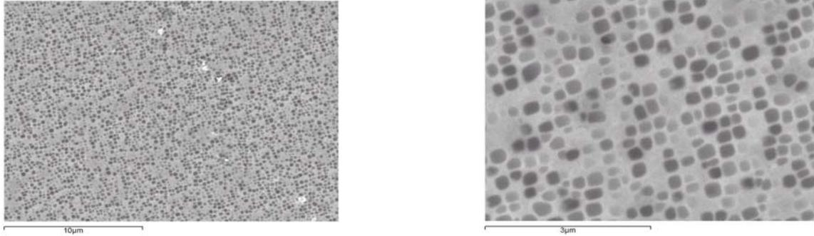
**Figure 6.** After heat-treatment at 1055°C/ 1 hr. (AC), and 845°C/ 24 hr. (AC); Condition No. 3
