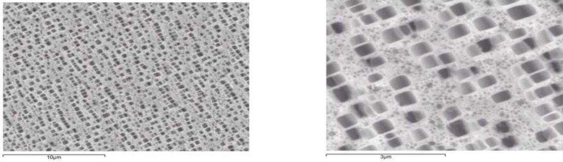
**Figure 8.** After heat-treatment at 1125°C/ 2hr. (AC), 925°C / 1 hr. (AC), and 845°C / 24 hr. (AC); Condition No. 5
