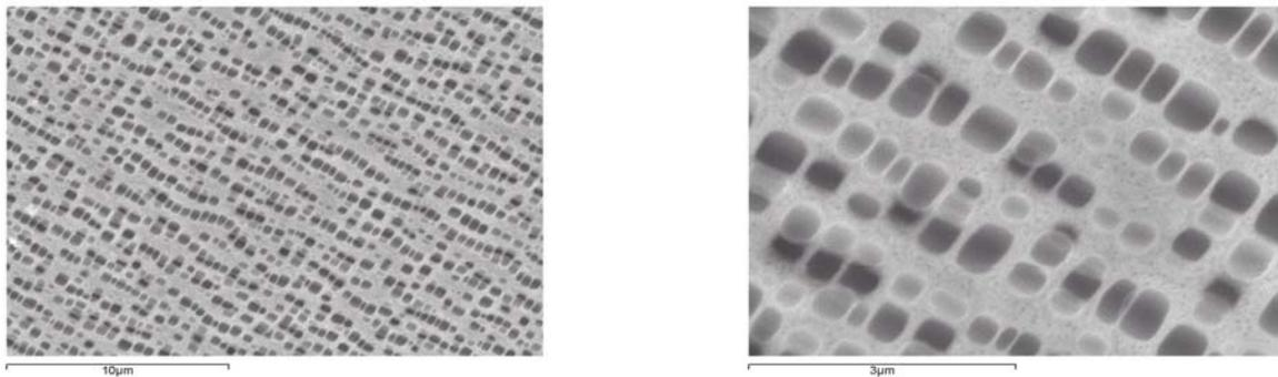
**Figure 7.** After heat-treatment at 1125°C / 2hr. (AC) and 845°C / 24 hr. (AC); Condition No. 4
