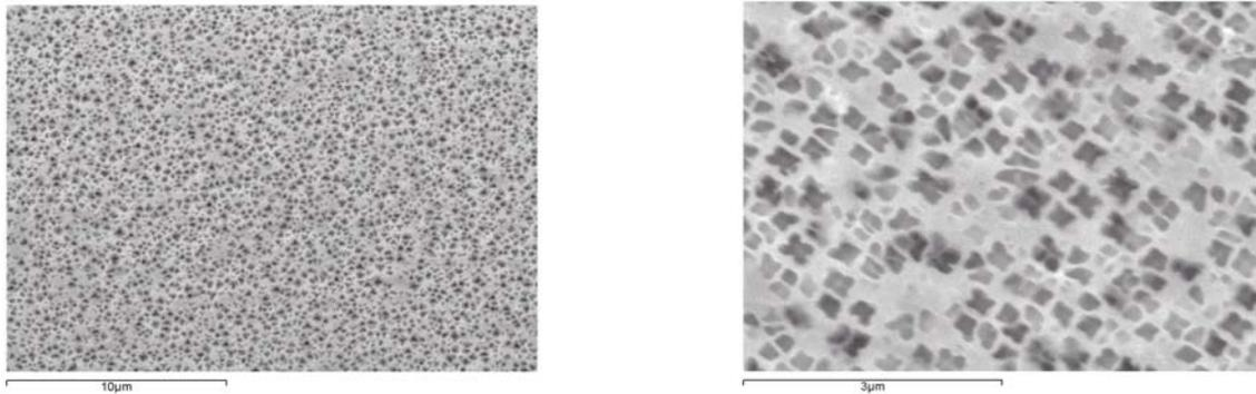
**Figure 4.** After heat-treatment at 845°C / 24 hr. (AC); Condition No. 1
