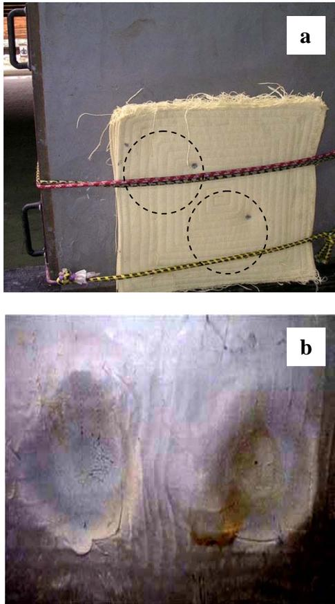
**Figure 4** Testing of 30 layers of aramid fabric with .44 magnum: (a) stop of the bullet in the Kevlar and (b) indentation of the modeling clay at the back of the aramid fabric.
