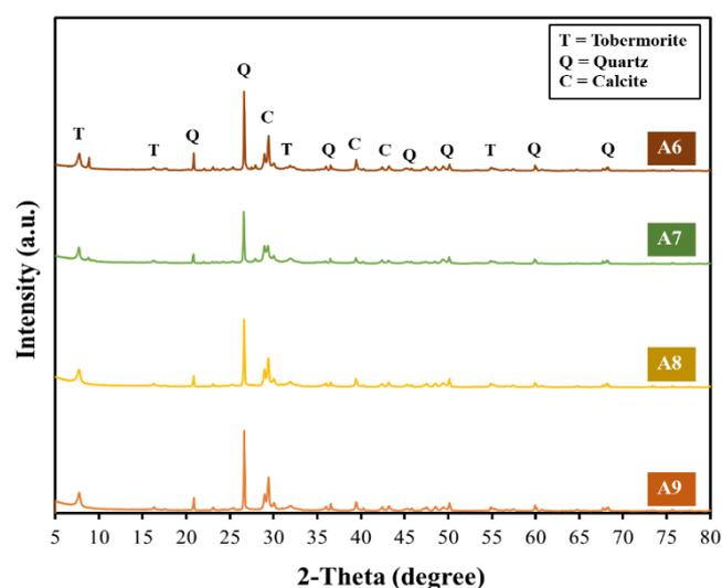
Figure 4. XRD patterns of lightweight concrete samples from A6 to A9.
