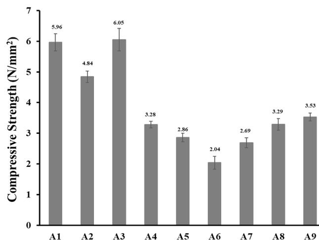
Figure 3. The compressive strength of lightweight concrete samples from A1 to A9.
