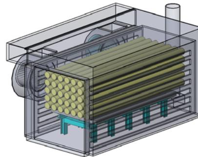
**Figure 1.** Model of stacking of billets in heating furnace.
