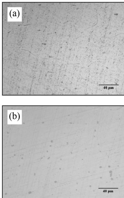
**Figure 6.** Microstructure of (a) as-cast billet contained  $\beta$ -AlFeSi and Mg<sub>2</sub>Si and (b) homogenized billet contained  $\alpha$ -Al(FeMn)Si. Mg<sub>2</sub>Si precipitates were dissolved.
