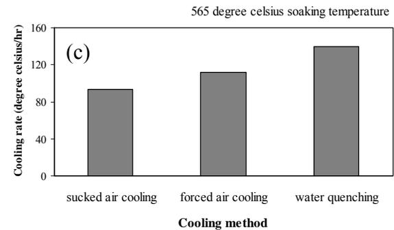
**Figure 4.** A summary of cooling rates of soaked billet at (a) 585°C, (b) 575°C and (c) 565°C with sucked air cooling, forced air cooling, and water quenching.
