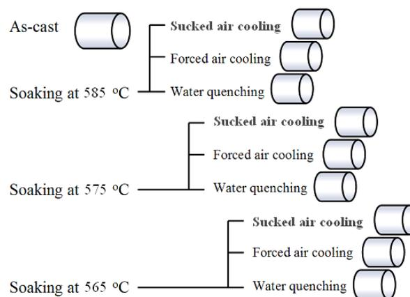
**Figure 2.** Conditions of specimens, i.e. as-cast and homogenizing at 585°C, 575°C and 565°C cooled by different methods.
