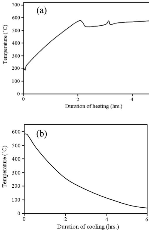
**Figure 3.** The relationship between temperature of aluminum billets and time during (a) homogenizing at 585°C and (b) cooling.
