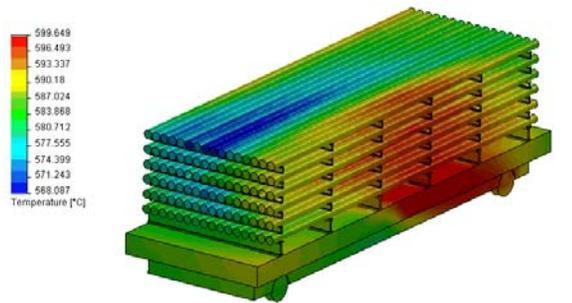
**Figure 5.** Temperature gradient of the stacking of billets during Homogenization analyzed by COSMOSFloWorks™.
