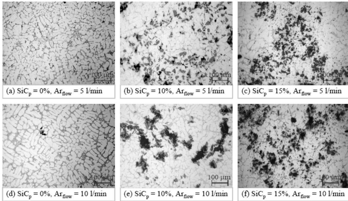
**Figure 3.** Microstructures at 680 °C casting temperature
