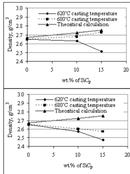
**Figure 4.** Density of  $\text{SiC}_p\text{-Al}$  composite
