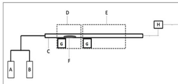
**Figure 1.** CVD set-up employed to synthesis aligned CNTs. A-Argon gas cylinder. B-Acetylene gas cylinder. C-Quartz tube. D - First heating furnace. E- Second heating furnace. F - Quartz boat. G-Controller. H- Water bubbler
