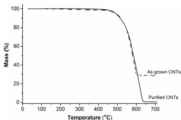
**Figure 5.** TGA analysis of as grown and purified aligned CNTs
