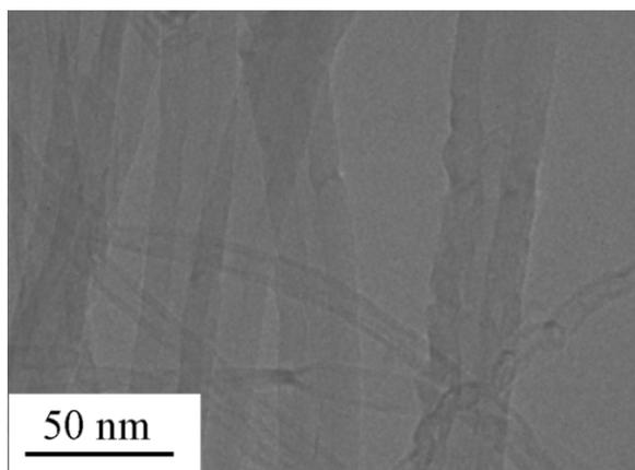
**Figure 3.** TEM Images of grown aligned CNTs
