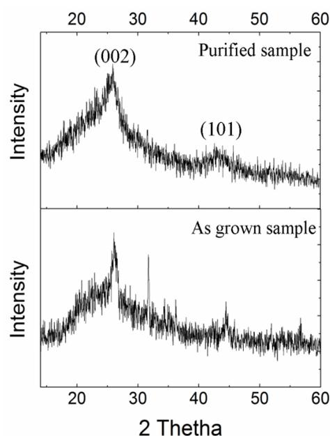
**Figure 6.** XRD peaks of as grown and purified sample grown
