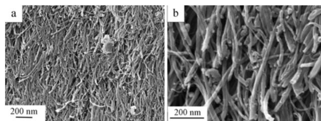
**Figure 2.** SEM Images (a) Low magnification (b) High magnification of grown aligned CNTs
