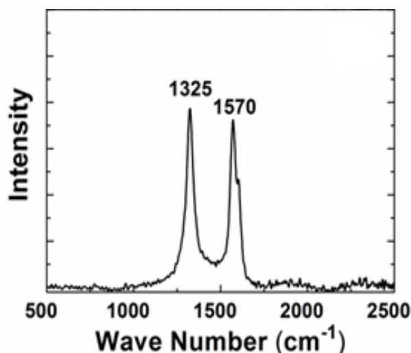
**Figure 4.** Raman spectra of grown aligned CNTs
