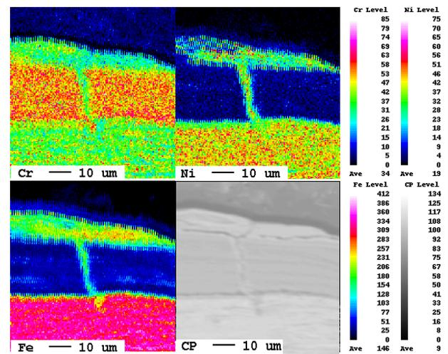
**Figure 6.** EPMA of cross-section of ring tested up to a distance of 576 m
