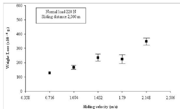
**Figure 4.** The relationship between weight loss of ring and sliding velocity
