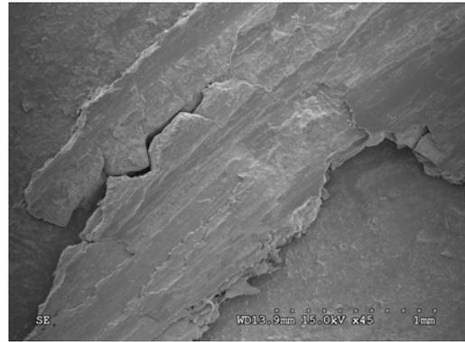
**Figure 2.** Stainless steel sticking on VC
