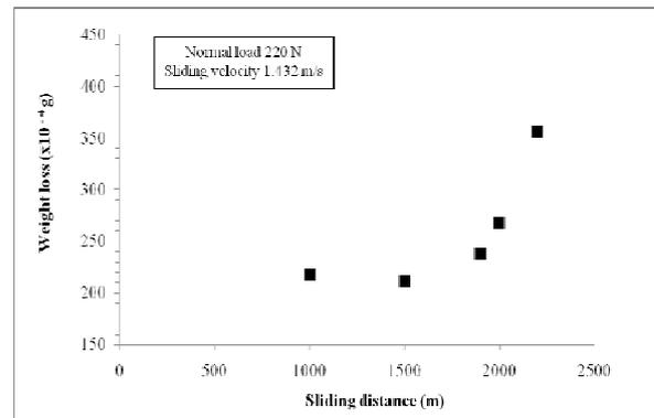
**Figure 3.** The relationship between weight loss of stainless steel ring and sliding distance
