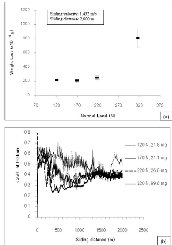
**Figure 5.** (a) The relationship between weight loss of ring and normal load, (b) friction coefficient during sliding test at various normal loads
