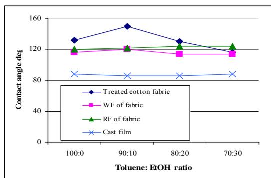
**Figure 1.** Contact angle of treated cotton fabric using toluene: EtOH solvent (WF = Wash-fastness; RF = Rub-fastness).
