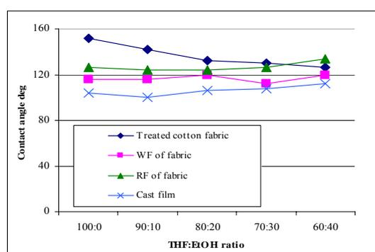
**Figure 2.** Contact angle of treated cotton fabric using THF:EtOH solvent (WF = Wash-fastness; RF = Rub-fastness).
