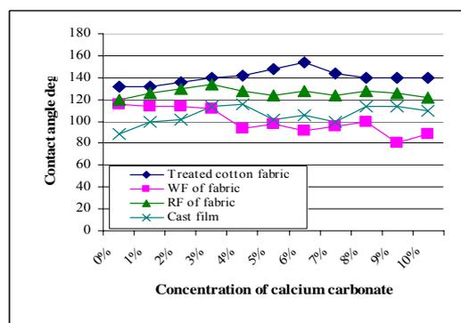
**Figure 4.** Contact angle of treated cotton fabric with adding calcium carbonate particles (WF = Wash-fastness; RF = Rub-fastness).
