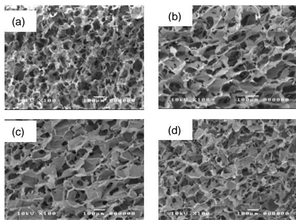
**Figure 4.** SEM micrographs of collagen/chitosan scaffolds at different blending composition: (a)100/0, (b)90/10, (c)70/30, and (d)0/100.
