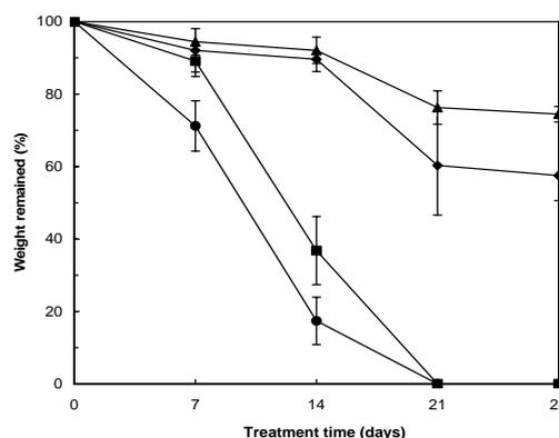
**Figure 5.** In vitro biodegradation of collagen/chitosan scaffolds with different blending compositions: (●) 100/0, (■) 90/10, (◆) 70/30, and (▲) 50/50 (collagen/chitosan).
