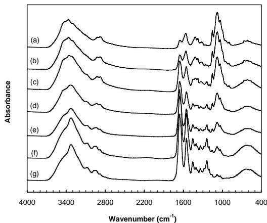
**Figure 1.** FT-IR spectra of collagen/chitosan scaffolds with different blending compositions : (a) 0/100, (b)10/90, (c)30/70, (d)50/50, (e)70/30, (f)90/10,and(g)100/0collagen/chitosan).
