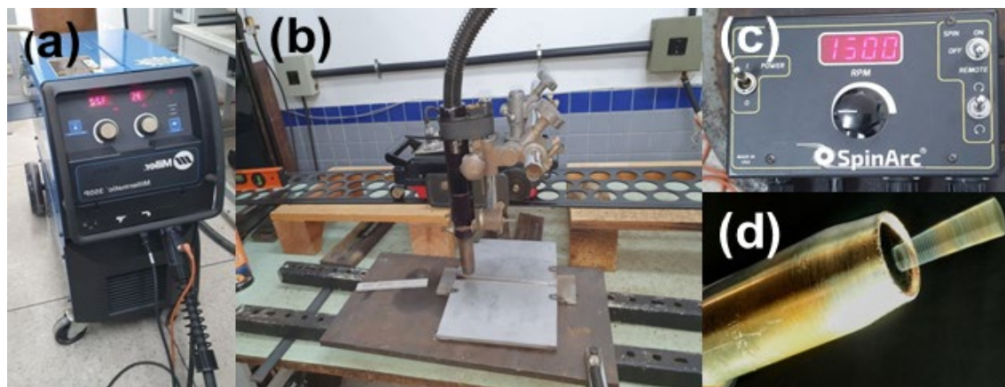
Figure 2. Apparatus for welding and visual aspect of the narrow gap joint. (a) welding machine; (b) assembling for welding; (c) frequency controller; (d) welding torch showing the rotating wire.
