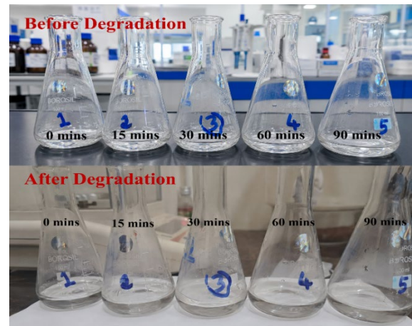
Figure 5. Photographs of photodegradation experiment of CIP in various time intervals before and after degradation.
