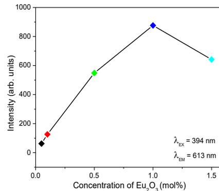
**Figure 6.** Relationship between the intensity of emission at 613 nm wavelength by excited 394 nm with the concentration of Eu<sub>2</sub>O<sub>3</sub>.
