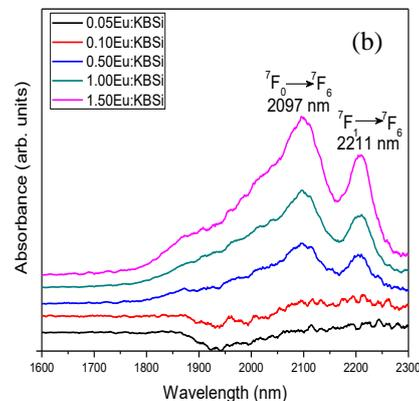
**Figure 3.** The Absorption spectra of the  $\text{KBSi:Eu}^{3+}$  glasses.
