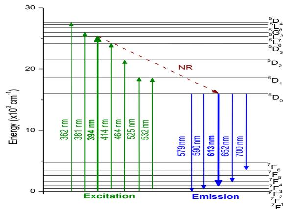
**Figure 7.** Energy level diagrams of Eu<sup>3+</sup> doped KBSi glasses.
