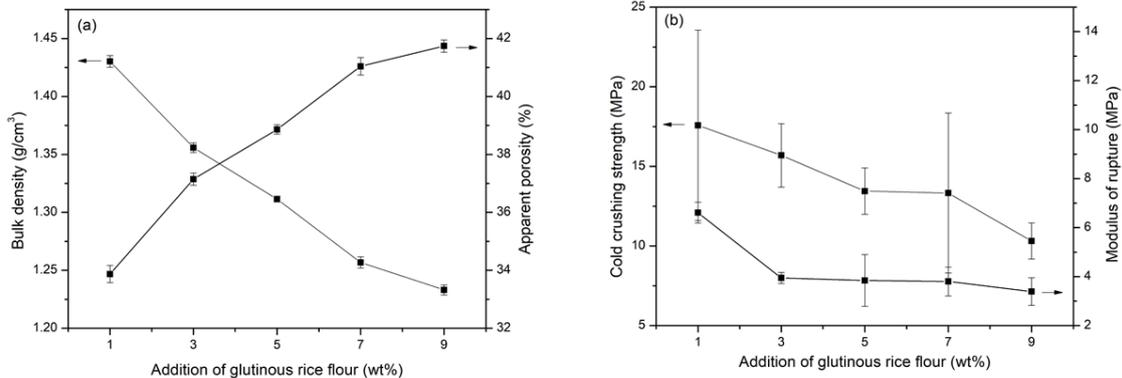
**Figure 9.** (a) Bulk density and apparent porosity and (b) cold crushing strength and modulus of rupture of the porous fused silica ceramics with glutinous rice flour addition sintered at 1150°C.
