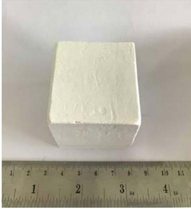
**Figure 2.** Photograph of fused silica ceramics sintered at 1150°C.
