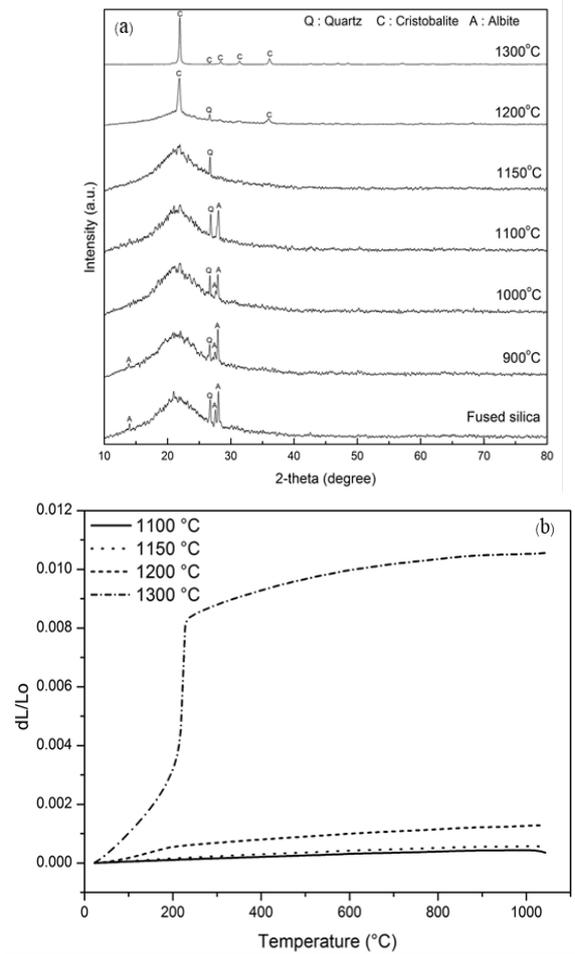
**Figure 8.** (a) XRD patterns, and (b) dilatometric curves of the fused silica ceramics sintered at different temperatures.
