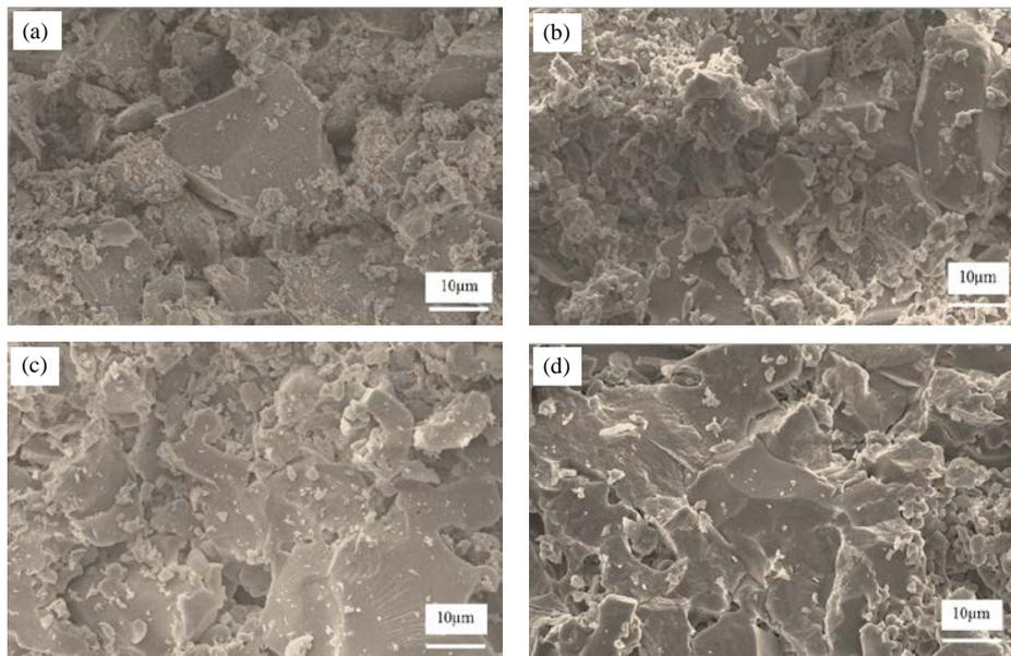
**Figure 7.** SEM images of the fused silica ceramics sintered at (a) 1100°C, (b) 1150°C, (c) 1200°C and (d) 1300°C.
