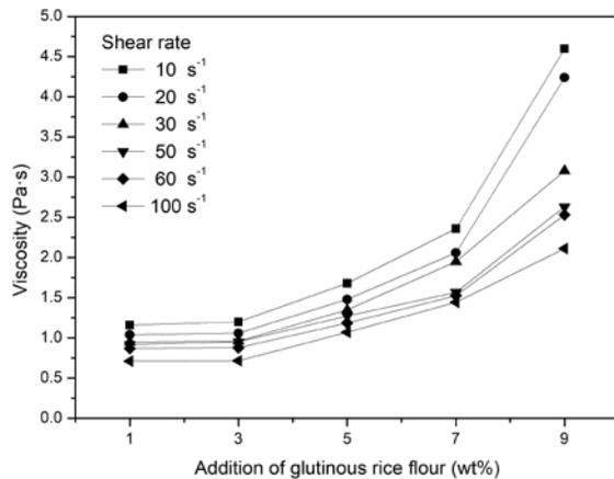
**Figure 3.** Rheological behavior of the fused silica slurries with different amounts of glutinous rice flour at room temperature.
