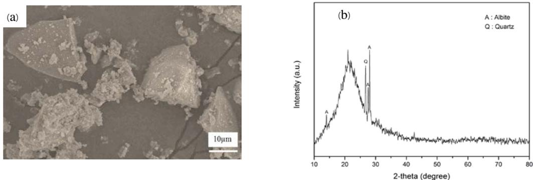
**Figure 1.** (a) SEM image, and (b) XRD pattern of the fused silica powder.
