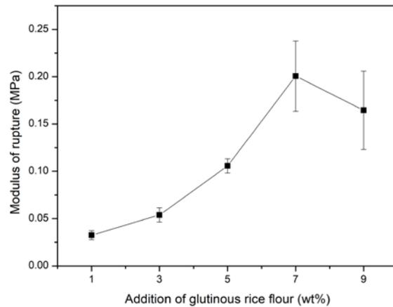
**Figure 4.** Modulus of rupture of the fused silica green samples with various glutinous rice flour addition.
