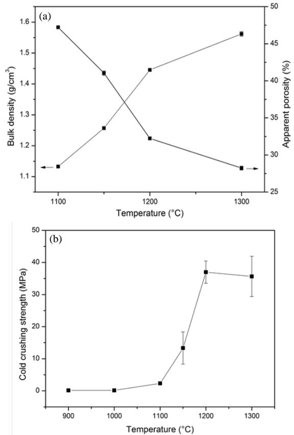
**Figure 6.** (a) Bulk density and apparent porosity and (b) cold crushing strength of the fused silica ceramics sintered at different temperatures.
