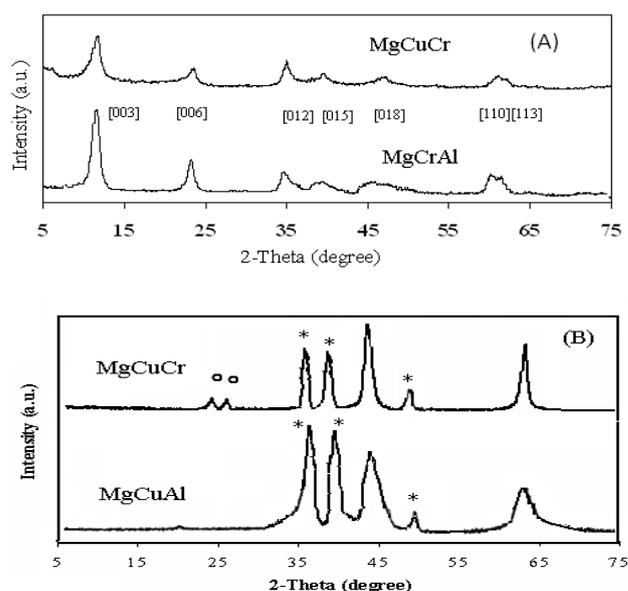
**Figure 3.** XRD patterns of (A) LDHs and (B) mixed oxides. (\*) CuO, (o)  $CuCrO_4$
