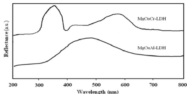
**Figure 5.** UV-vis diffuse reflectance spectra of MgCuAl-LDH and MgCuCr-LDH.
