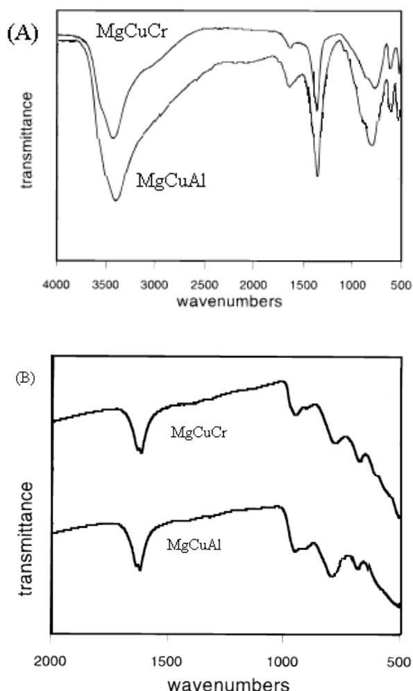
**Figure 4.** FTIR spectra of (A) LDHs and (B) mixed oxides.
