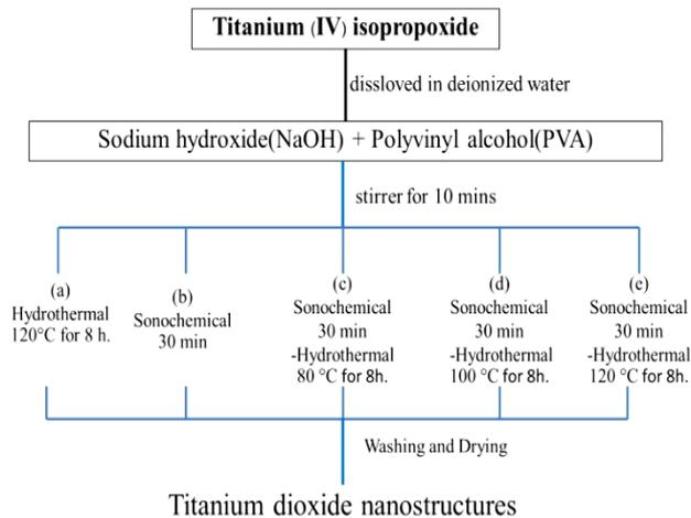
**Figure 1.** Flow chart of the sonochemical-hydrothermal process.
