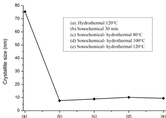
**Figure 3.** The grain size of  $\text{TiO}_2$  synthesized by sonochemical-hydrothermal process.
