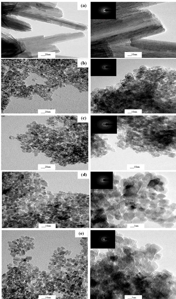
**Figure 5.** TEM images of TiO<sub>2</sub> nanoparticles synthesized by (a) hydrothermal at 120°C, (b) sonochemical for 30 minutes, (c) sonochemical-hydrothermal at 80°C, (d) sonochemical-hydrothermal at 100°C, (e) sonochemical-hydrothermal at 120°C.
