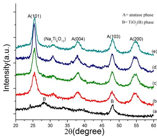
**Figure 2.** XRD patterns of  $\text{TiO}_2$  nanoparticles synthesized by (a) hydrothermal at  $120^\circ\text{C}$ , (b) sonochemical for 30 min, (c) sonochemical-hydrothermal at  $80^\circ\text{C}$ , (d) sonochemical-hydrothermal at  $100^\circ\text{C}$ , (e) sonochemical-hydrothermal at  $120^\circ\text{C}$ .
