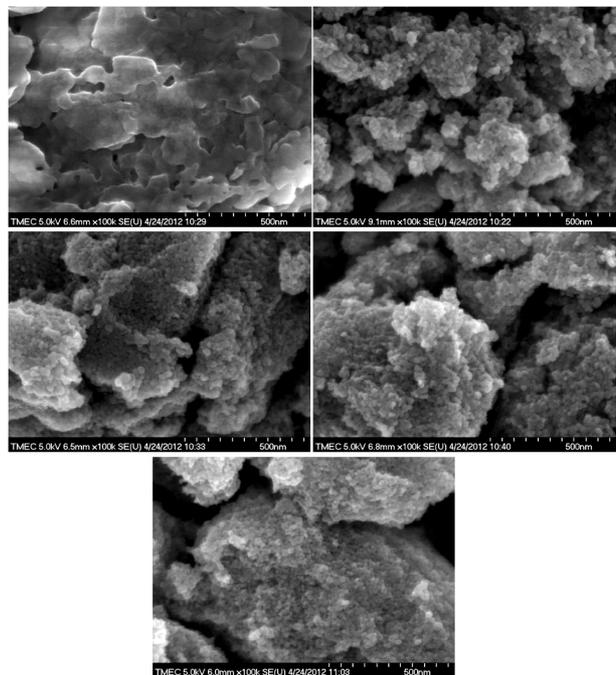
**Figure 4.** FE-SEM images of  $\text{TiO}_2$  nanoparticles synthesized by (a) hydrothermal at  $120^\circ\text{C}$ , (b) sonochemical for 30 min, (c) sonochemical-hydrothermal at  $80^\circ\text{C}$ , (d) sonochemical-hydrothermal at  $100^\circ\text{C}$ , (e) sonochemical-hydrothermal at  $120^\circ\text{C}$ .
