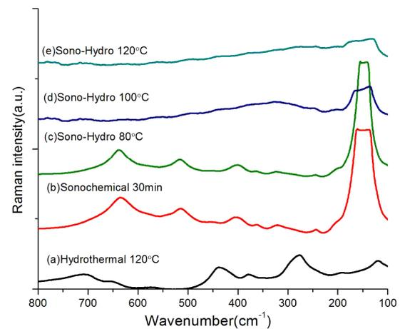
**Figure 6.** Raman spectra of TiO<sub>2</sub> nanoparticles synthesized by (a) hydrothermal at 120°C, (b) sonochemical for 30 minutes, (c) sonochemical-hydrothermal at 80°C, (d) sonochemical-hydrothermal at 100°C, (e) sonochemical-hydrothermal at 120°C.
